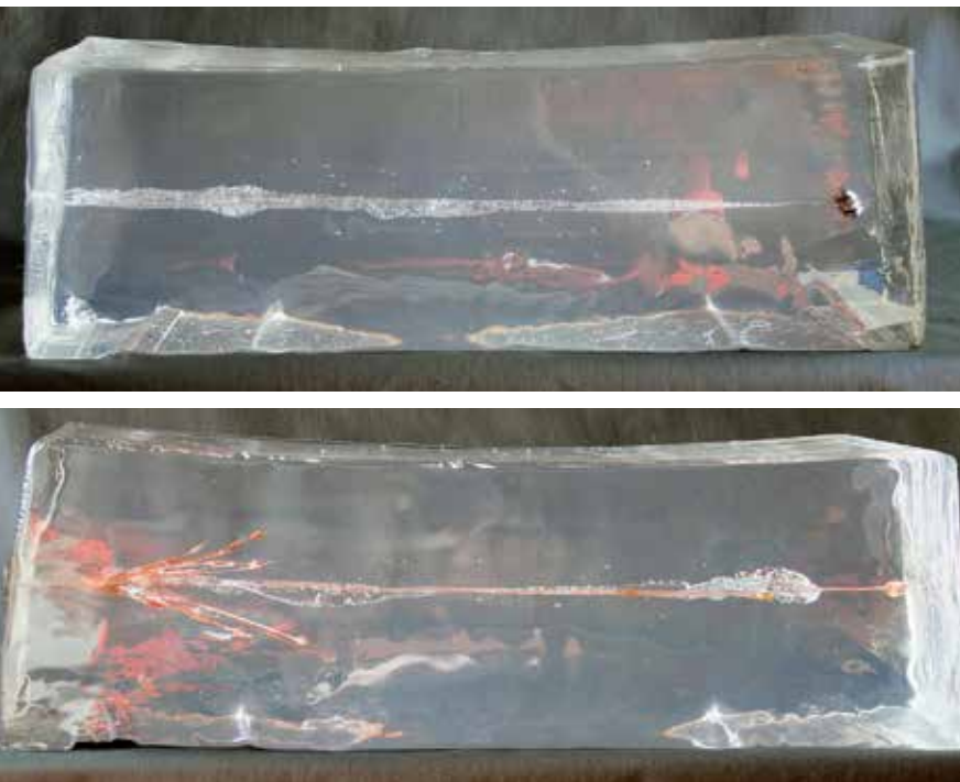
ABOVE: Though demonstrating considerably more terminal ballistic effect in a 6-by-6-by-16-inch block of ballistic gelatin than a traditional 9mm JHP (top), the DRT 85-grain Terminal Shock JHP (bottom) penetrated just as far.
