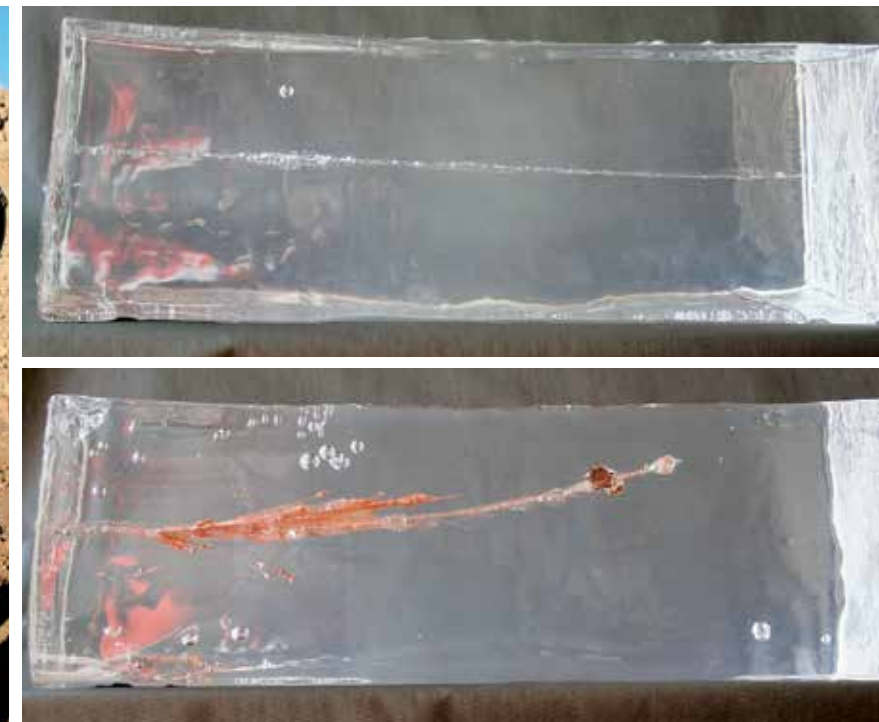
ABOVE: FBI testing in ballistic gelatin shows that a standard 230-grain .45 ACP JHP (top) failed to expand despite deep penetration. However, DRT's 150-grain Terminal Shock JHP (bottom) demonstrated tremendous effect and still penetrated about 12 inches.
