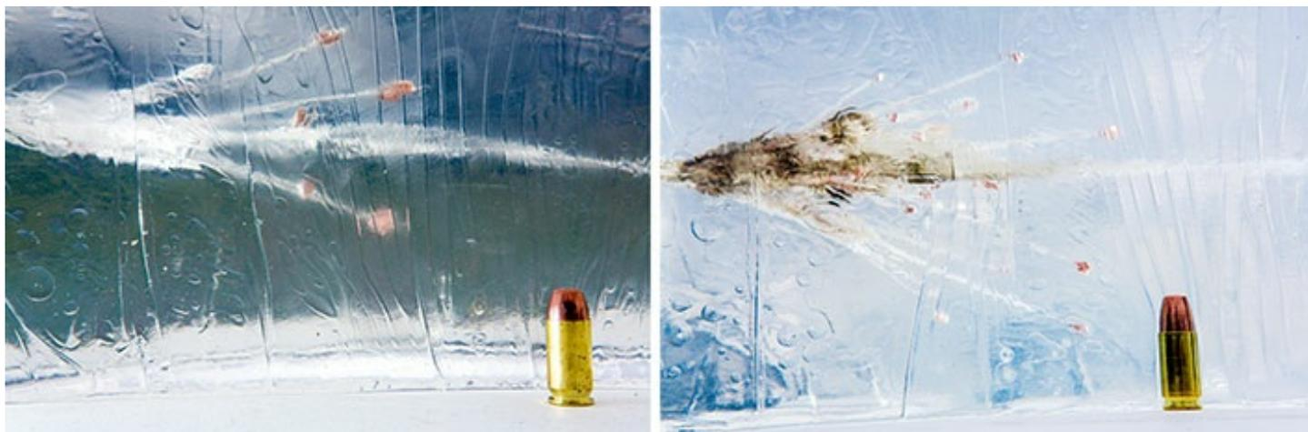
DRT Terminal Shock penetrates semi-hard barriers and begins to break up in soft targets as seen above in ballistic gelatin. A .45 ACP round is shown at top and a 9 mm round appears in the bottom image.
