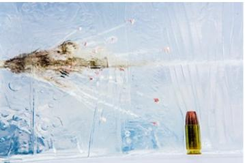
DRT Terminal Shock penetrates semi-hard barriers and begins to break up in soft targets as seen above in ballistic gelatin. A .45 ACP round is shown at top and a 9 mm round appears in the bottom image.
